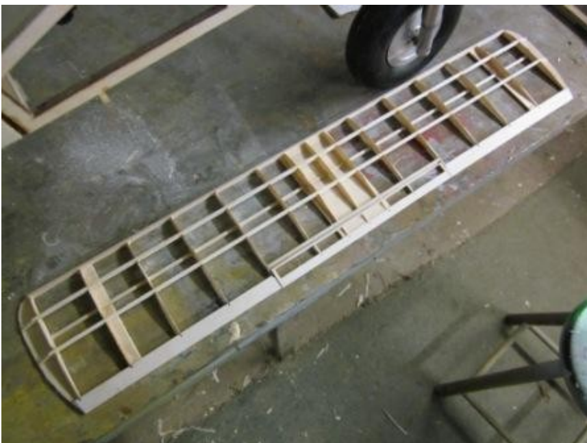
Stabiliser and elevator are next in line and all up weighed 19g. Elevator will work with a fishing line pull-pull system to a micro servo
