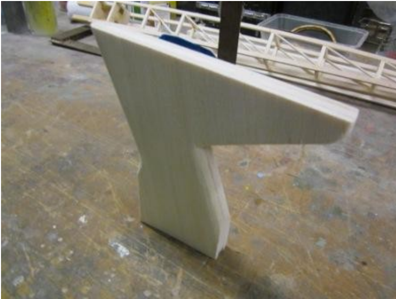
This is the wing mount pylon made from cross grained 4mm balsa sheet over a 4mm frame.
