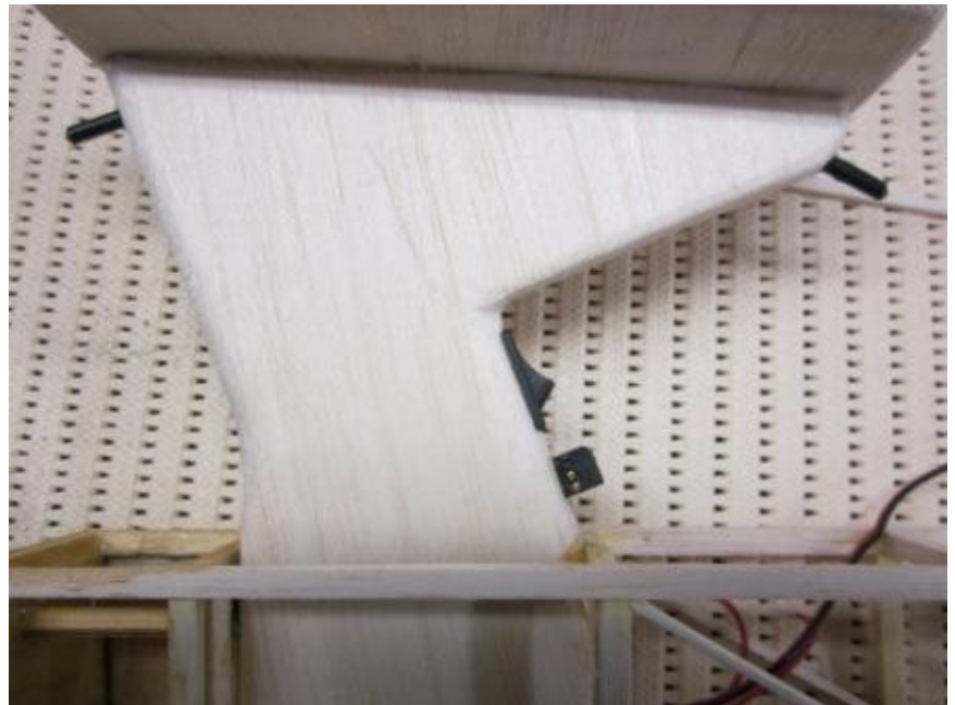
The 2 x 2 Eneloop AAA 750mah batteries are fitted either side of the pylon.
